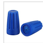
Waterproof Wire Nuts - Medium (Fits 14AWG - 22AWG, up to 3 wires of 16/2)
